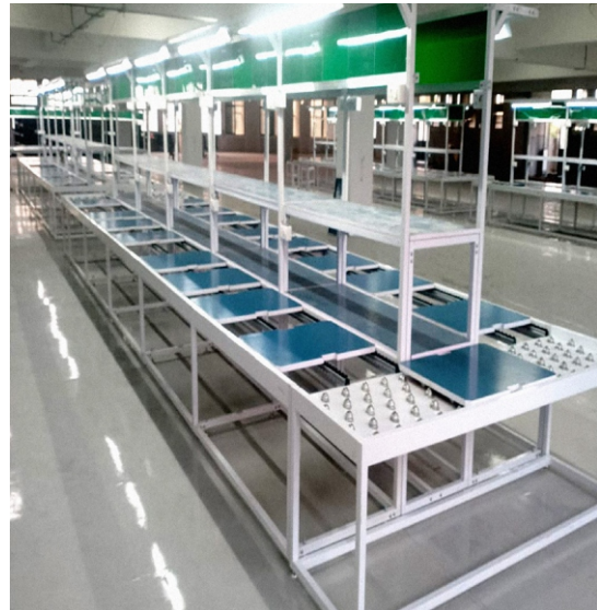
FINAL ASSEMBLY MANUAL FREE FLOW CONVEYOR WITH BALL TRANSFER TABLE
