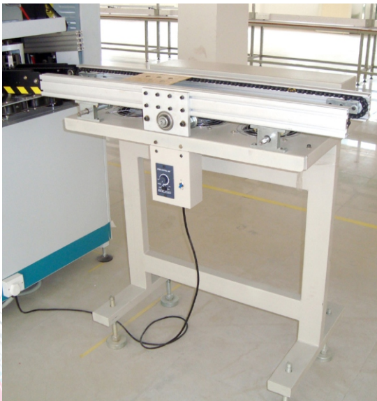
INPUT CONVEYOR FOR WAVE SOLDERING SINGLE SIDED
