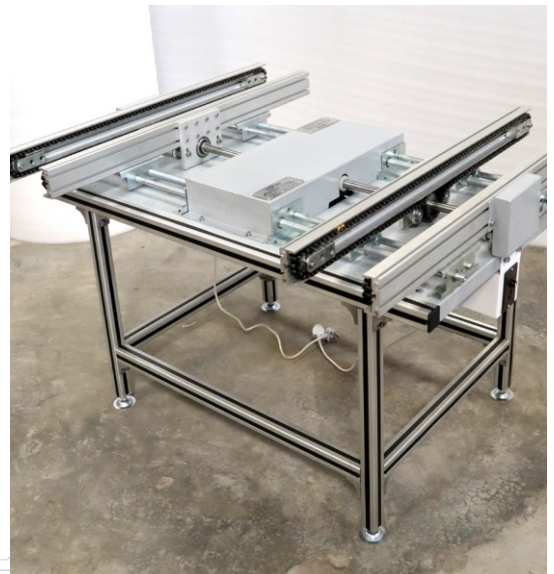
INPUT CONVEYOR FOR WAVE SOLDERING DOUBLE SIDED
