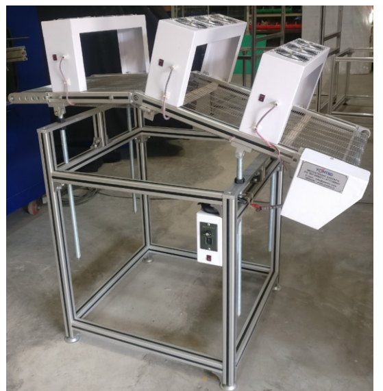
OUTPUT WAVE COOLING CONVEYOR SS MESH BELT
