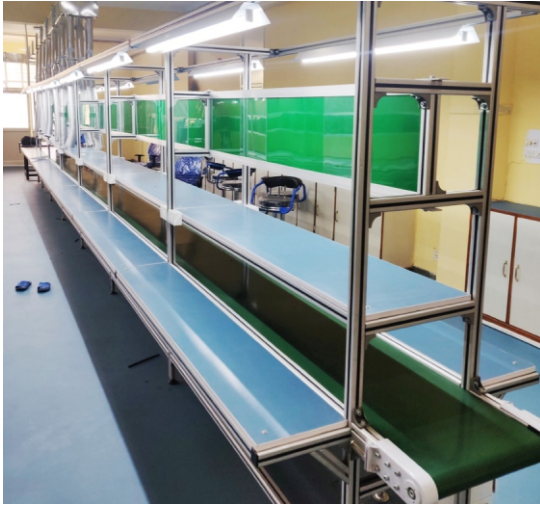
FINAL ASSEMBLY MOTORISED FREE FLOW CONVEYOR
