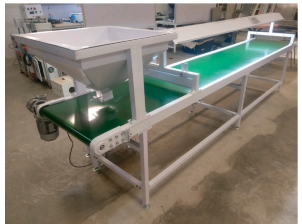
Sorting Conveyor with Hopper
